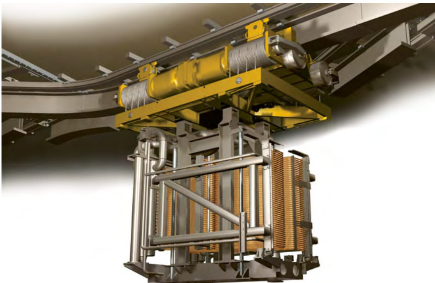
View of NB calorimeter during transportation by the neutral beam remote handling system monorail crane
