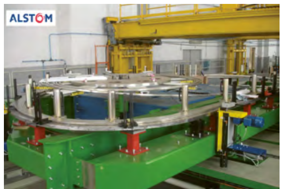
Winding line with the first wound single pancake at Alstom
