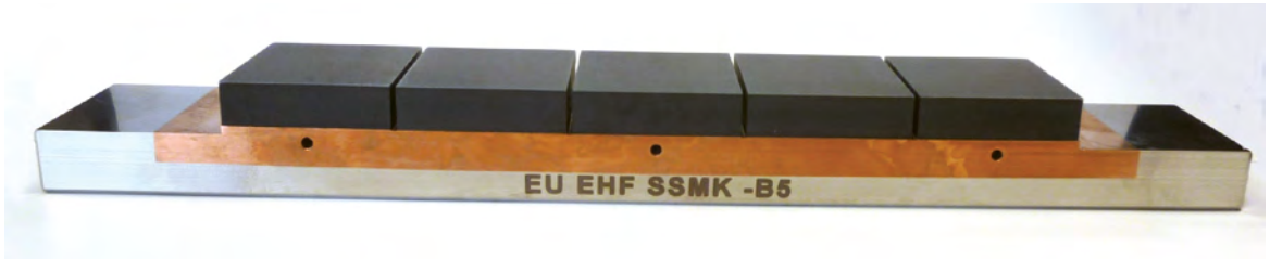
Small scale mock-up of the ion cyclotron resonance Faraday shield (courtesy of Atmostat)
