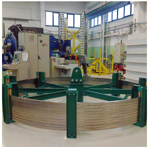
The 100m superconducting poloidal field qualification conductor length on its transportation jig
