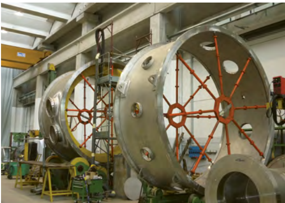
SPIDER vacuum vessel manufacturing at Zanon premises.
