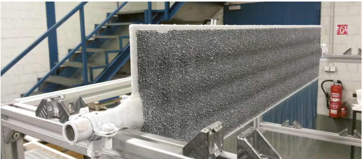
A pre-production cryopump cryopanel after charcoal spraying and a cold test at 77K (courtesy of KIT)
