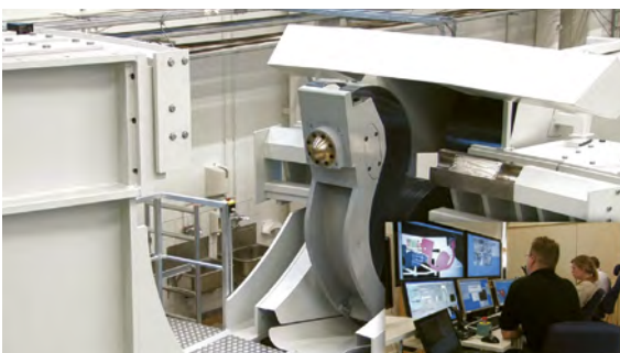
Remote Handling trials being conducted at DTP2 test facility
