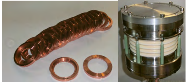
Copper rings for the gyrotron beam tunnel and body ceramic insulator for the 1MW short pulse gyrotron (F4E-OPE-458)
