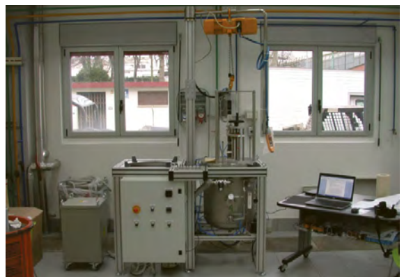
Equipment to measure erosion/corrosion in SiC/SiC with liquid metals
