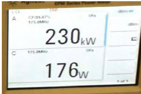
Experimental arrangement in the joint performance tests for the final power amplification stages of the RF power system provided by CIEMAT and observation of target output power level of 230 kW.
