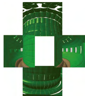
Schematic composite of the four different views of the ITER plasma facing components provided by the equatorial visible/infra-red wide angle viewing system from one of the equatorial port plugs
