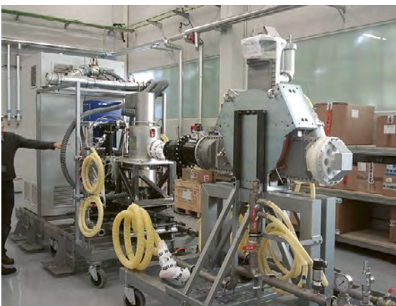
The Li Target Assembly prototype set up and used for the RH studies
