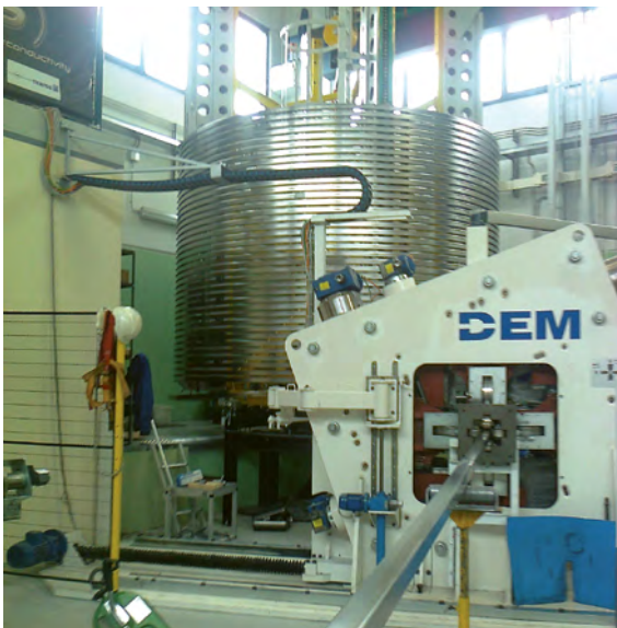
Fabrication of the first poloidal field copper dummy length at Criotec (compaction and spooling)
