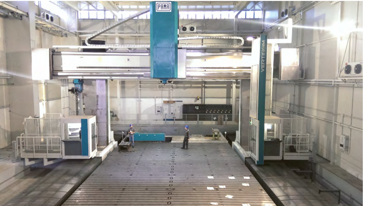
Portal milling machines for the production of 70 radial plates (courtesy of CSC)
