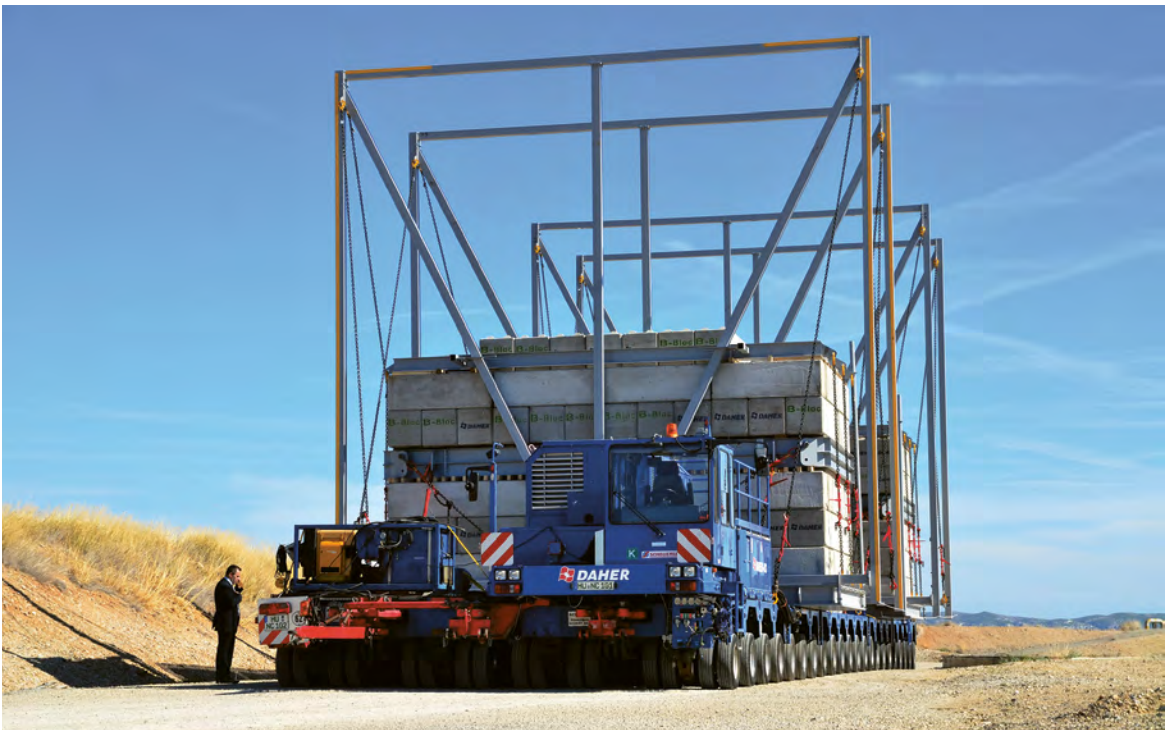
The ITER Test Convoy: 800 tonnes on 352 tyres crossing the South of France
