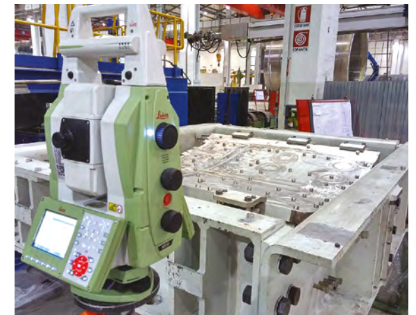
PS1 mock up under dimensional inspection.
