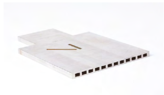
Full-scale or near full-scale mock-ups of TBM sub-components realised with standardised welding procedure specifications: (Top left) HCLL cooling plate; full size (ATMOSTAT/CEA); (Top right) HCPB cooling plate; full-size (KIT); (Bottom right) TBM Box Side Cap; half-size (ATMOSTAT/CEA). Meandering channels for heat extraction in their thickness are constructed by mixed laser/diffusion-bonding or spark erosion/bending processes; tolerances achieved are the reference ones for TBMs.
