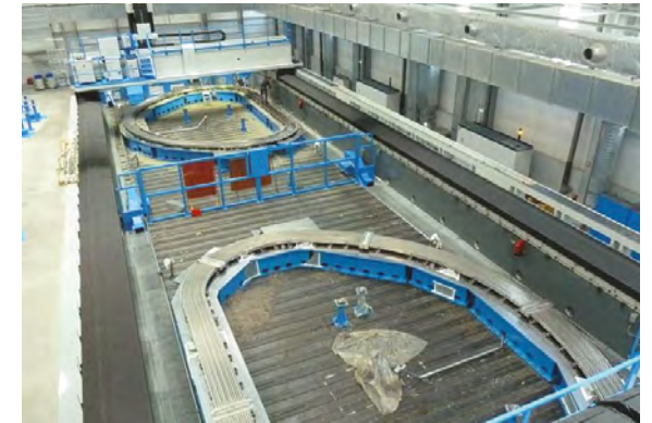
Machining of two radial plates by CNIM (courtesy of CSC)
