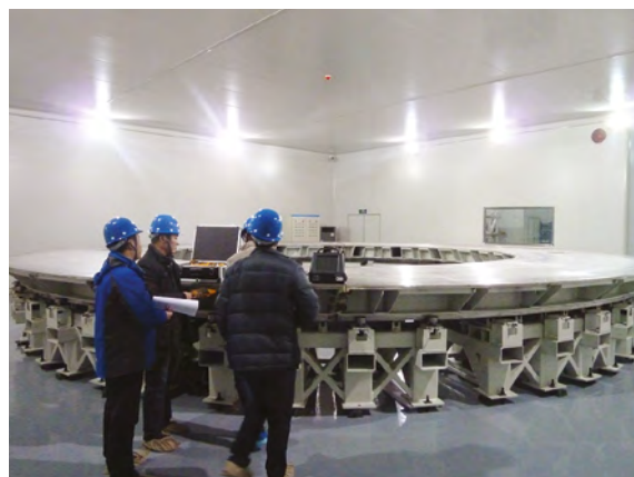
View of the poloidal field PF6 winding tooling line turntable during commissioning
