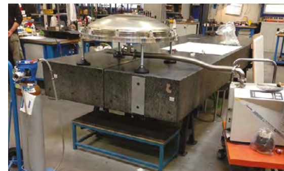
A cryopump thermal shield undergoing cold shock tests (courtesy of RI/SDMS)
