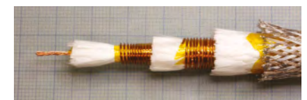
Internal structure of the Continuous External Rogowski coils (prototype)
