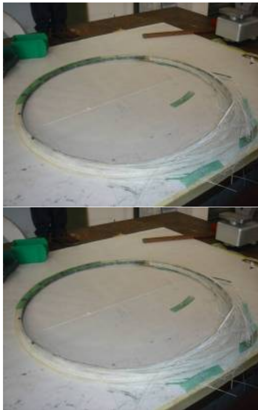
Figure 18 - Pre-compression ring mock-up after rupture
