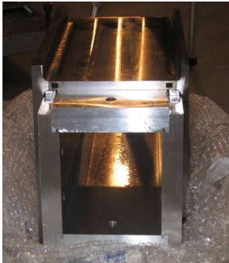
Figure 51 - Assembly mock-up of the TBM internal stiffening grid obtained by single-pass YAG laser welding of 11mm thick plates
