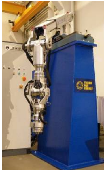
Figure 27 - Manipulator arm in a test stand in DTP2
