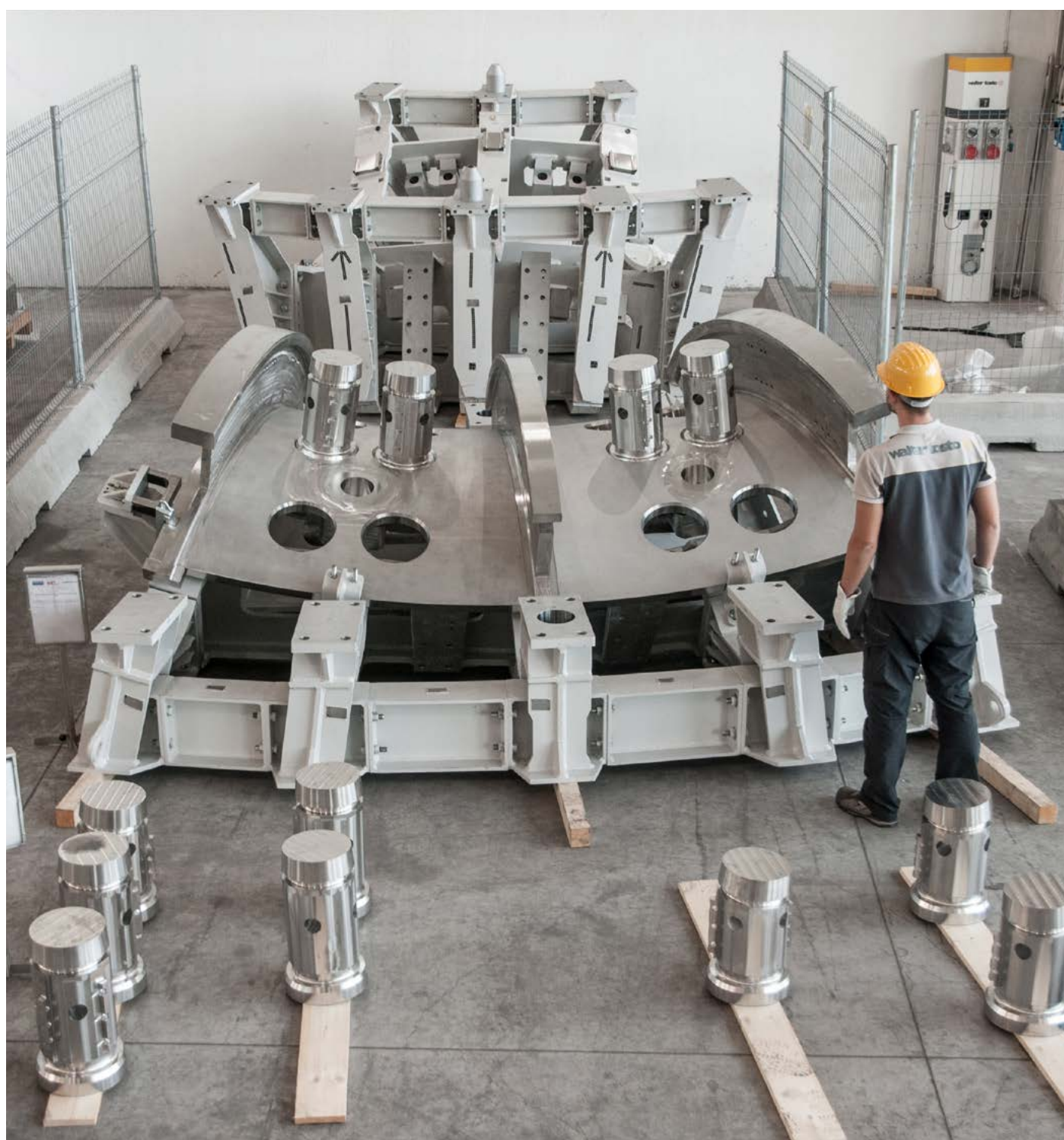
The ITER Vacuum Vessel is taking shape - October 2016 © Walter Tosto Spa
