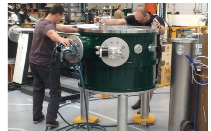
The magnet which will be joined to the gyrotron prototype and tested at SPC.
