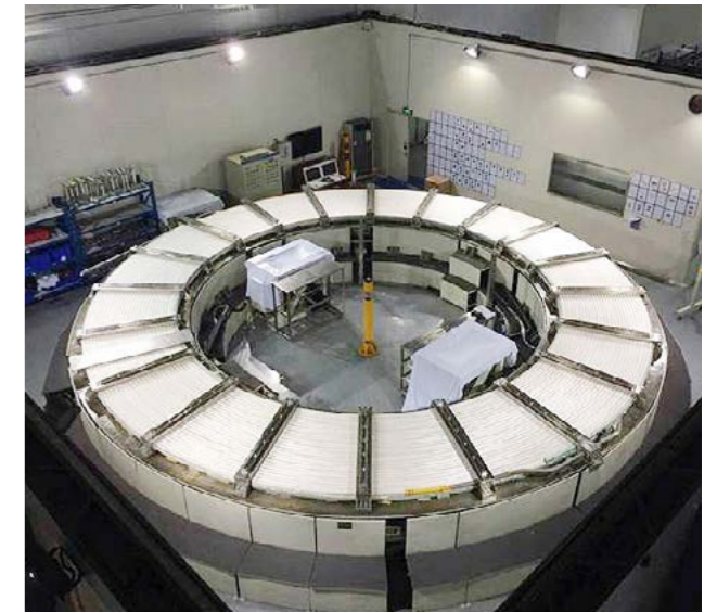
The dummy double pancake completed, ASIPP, China
