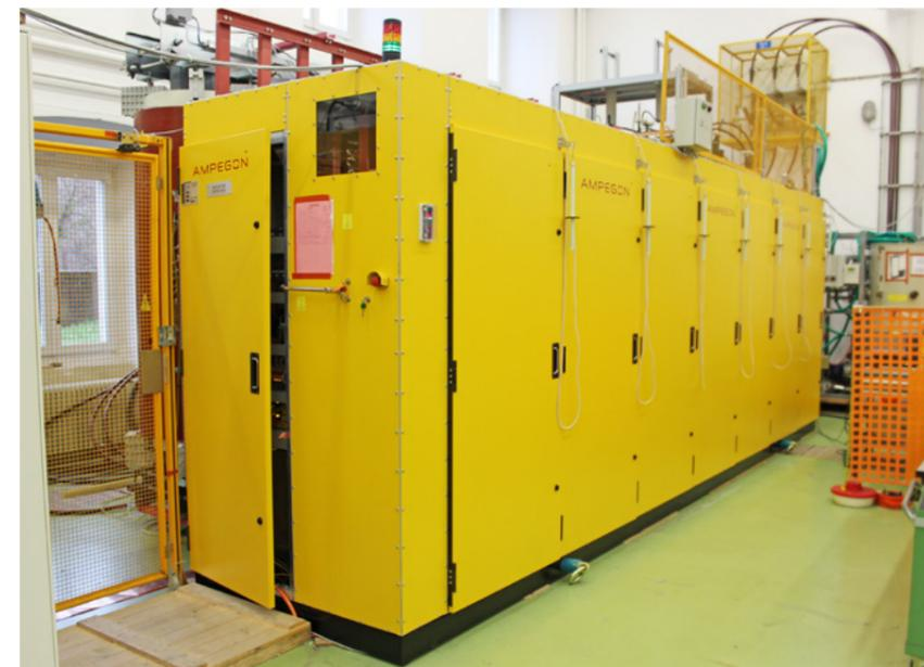
High voltage power supply unit financed by F4E and manufactured by Ampegon © F4E
