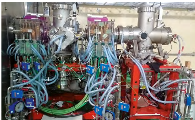
Low Energy Beam Transfer installed in Rokkasho, Japan
