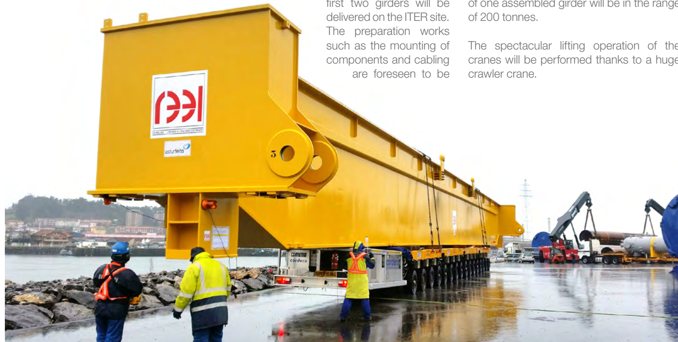
One of the four girders manufactured to support the 2 x 750 tonnes crane that will be installed in the Assembly Hall building. F4E – NKM/Reel ©
