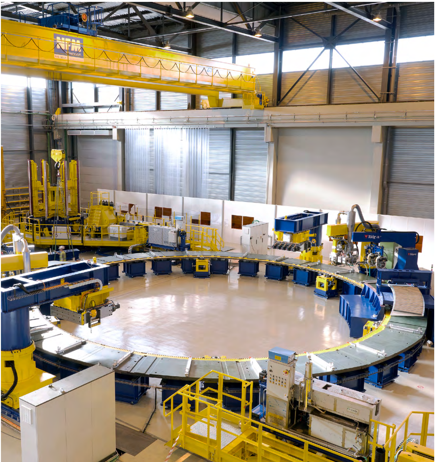
Setting up the conductor winding tooling station, ITER PF Coils facility, Cadarache.
