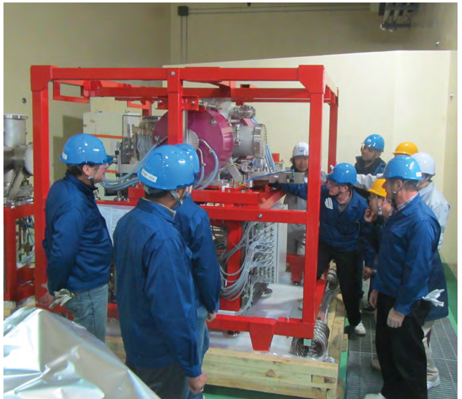
Preparing the low energy beam transport for vacuum testing
