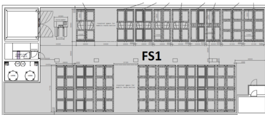
Figure 21 : TAPB2 - Preliminary Fire sectorization of the basement (B1)
